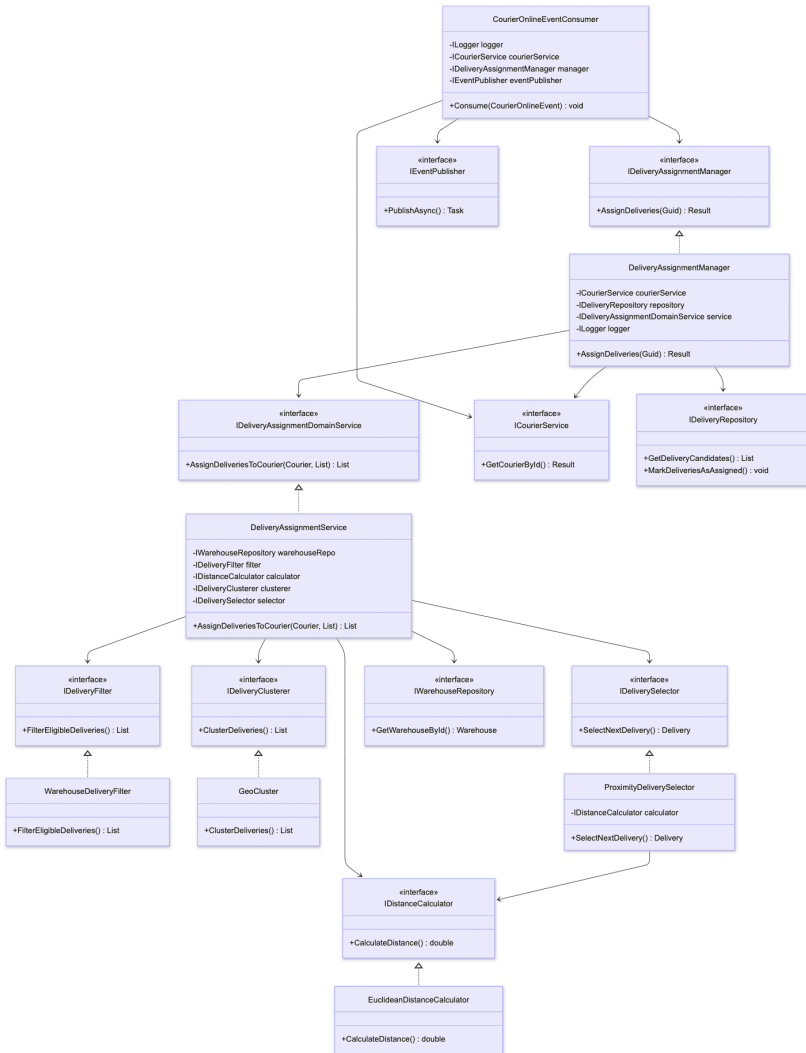
Figure 5.2: UML class diagram of the Delivery Assignment feature developed using TDD in this booklet
